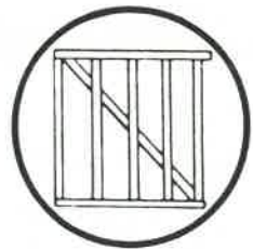
16" On Center Studding with Storm Bracing
