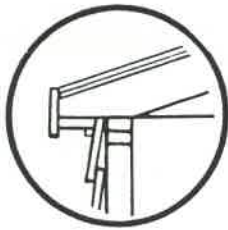
6" Boxed In Overhang on Eaves and Gables Protects Siding and Enhances appearance
